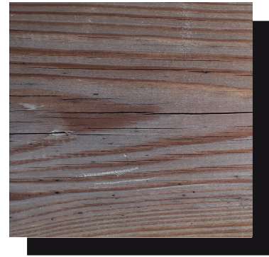
Old wood: after more than 1 year
